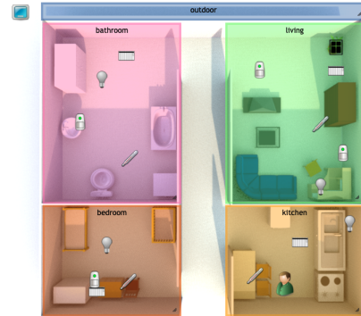
Fig. 8: The iCasa GUI showing the basic setup for our experiments: four rooms equipped with a presence sensor triggering heating and lighting, and a thermometer.
