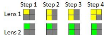
Fig. 3: Two Glider Lenses: map 3x3 cell patches from bottom lens to 1 higher cell in higher lens. Higher cell is live if the number of live cells in the lower patch is higher or equal to a threshold, which equals 1cell for Lens1 and 2cells for Lens2
